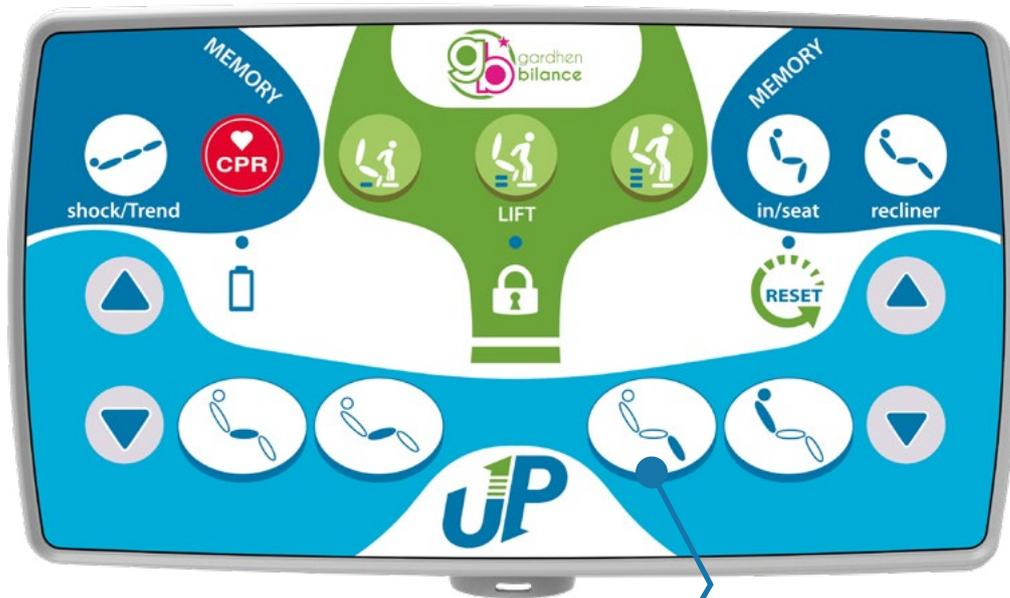
**BUTTON FOR THE MOVEMENT OF THE LEG SECTION**
